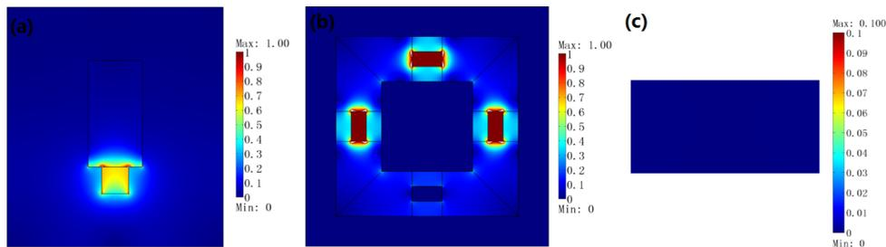
FIG. 6. FEM simulation results: the absolute value of the magnetic flux density distribution (a) when we replace the MH (with a relative permeability of 0.001 along the  $x$  direction and 1000 along the  $y$  direction) in Figure 1(a) with a high permeability material with a relative permeability of 1000; (b) when we replace the MH in Figure 2(b) by a high permeability material with a relative permeability of 1000; (c) We plot the DC magnetic field in the central air region of (b).
