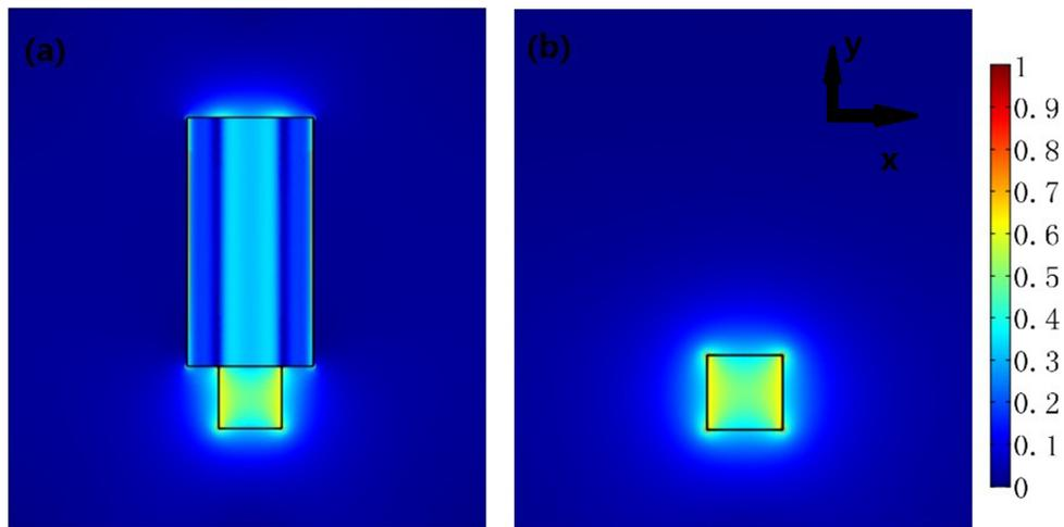
FIG. 1. FEM simulation results: the absolute value of the magnetic flux density distribution for (a) a magnet with a residual induction  $B_r = 1\text{T}$  in the  $y$  direction at the bottom of an MH with main axis along the  $y$  direction, and (b) only a single magnet with a residual flux density  $B_r = 1\text{T}$  in the  $y$  direction.
