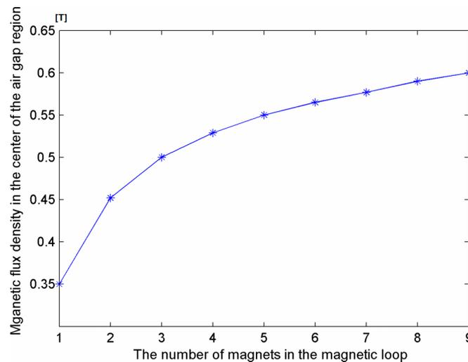
FIG. 3. The relation between the number of magnets in a single magnetic loop and the DC magnetic flux density in the center of the air region in the loop.
